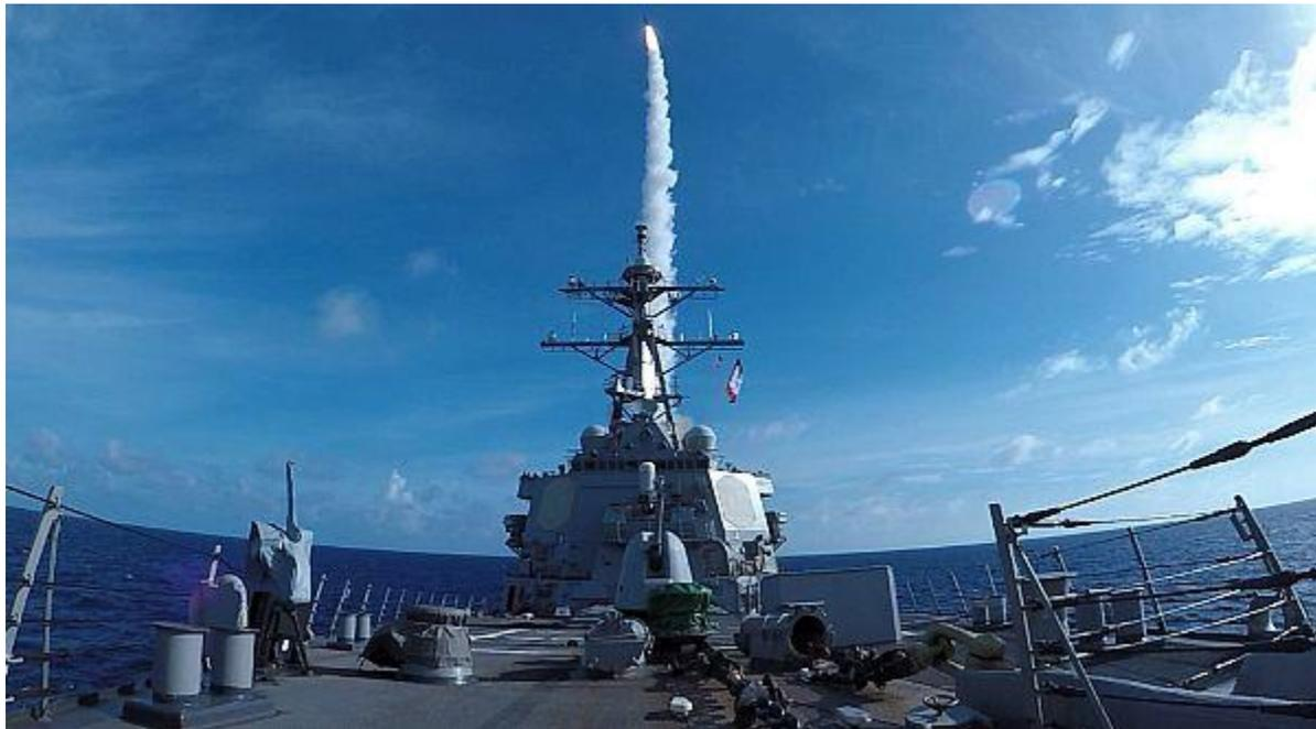
The missile exercise demonstrated The Sullivans' ability to defend against a close-in aerial attack. A BQM-74E air-launched drone served as the target. The ship successfully demonstrated its ability to employ a layered defense construct to engage a target with both the Mk 45 MOD2 (5"/54) caliber gun weapons system and the Aegis Weapons System.
